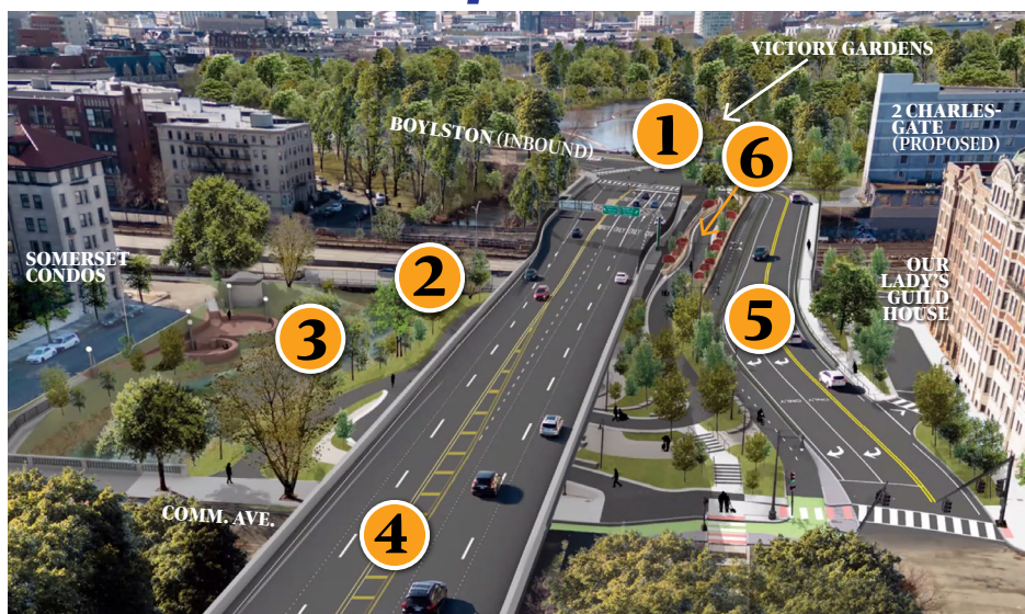
This rendering shows six key changes resulting from reconstruction of the Bowker Overpass. 1) Safer and simplified intersection of the Bowker and Boylston Street. 2) Removal of the existing exit ramp to Comm. Ave. 3) Additional trees and park landscaping along the Muddy River. 4) The rebuilt deck, which will have no sidewalks. 5) New on- and off-ramp, with a wide, ADA-compliant sidewalk. 6) New ped/bike ramp connecting Charlesgate and the Fens. (The view is from above Comm. Ave. looking toward the Victory Gardens.)
